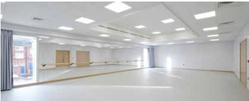
The dance studio has a sprung floor and a ceiling recess in the middle for high ballet lifts
